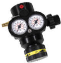
PRESSURE REGULATOR Piston Type 5,500-0 psi / 379.2-0 bar CGA 347/346 inlet Net Weight: 3.6lb 1.6kg Part No. 22-895401G2
