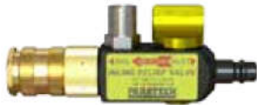
INLINE RELIEF VALVE FOR G2 165 psi / 11.4 bar Designed to relieve over-pressurization and allow a lift bag to remain inflated under a load. This valve will relieve excess pressure from an inflated bag caused by load shifts or temperature changes. Now with safety coupling. Net Weight: 1.0lb 0.4kg Part No. 22-890490-150
